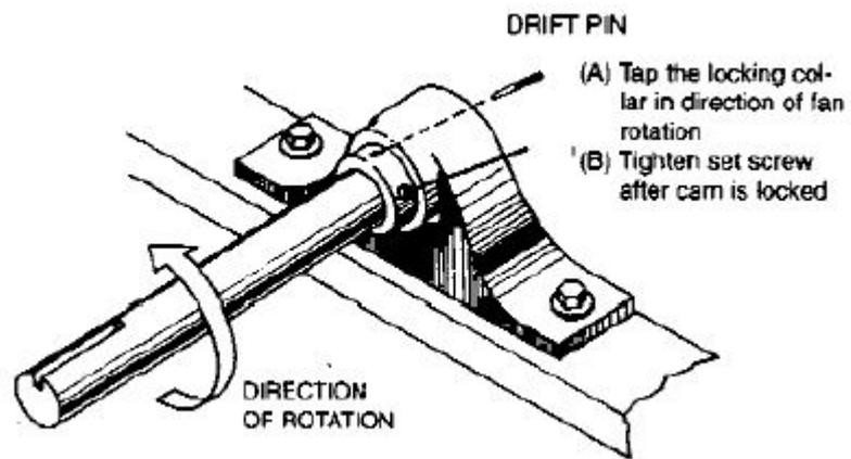
Figure 4. Locking Collar Assembly
