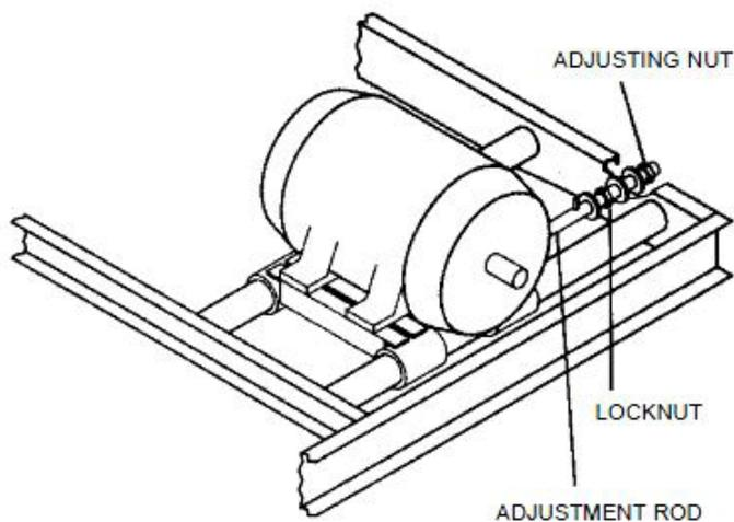
Figure 5. Adjustable Motor Base
