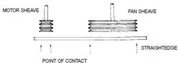
Figure 7. Checking Sheave Alignment
