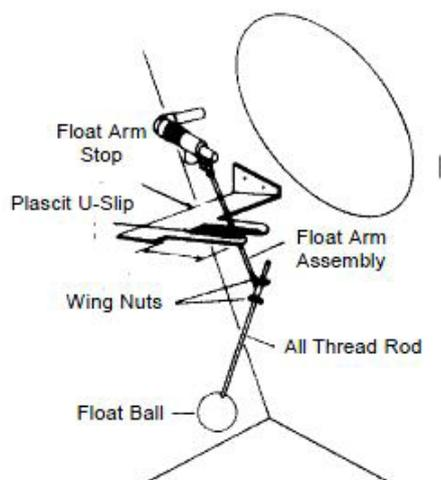
Figure 1. Water Make-Up Valve Assembly
